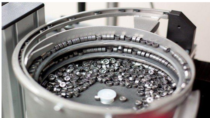
Figure 2 Vibratory Bowl Feeder
