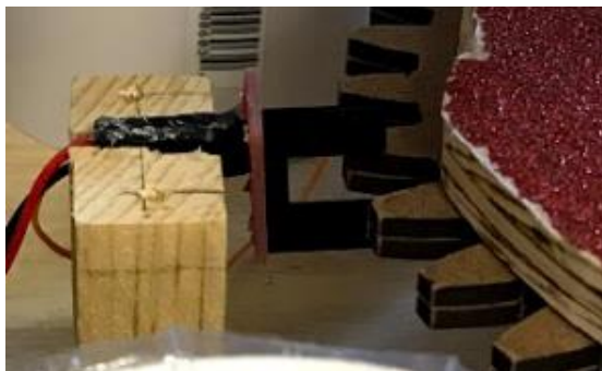
Figure 34 IR Interrupter mounting. This sensor is used for counting the angular position of the turntable. Similar to white tape sensor, the break beam sensor is inserted tightly into a slot of the vertical support.
