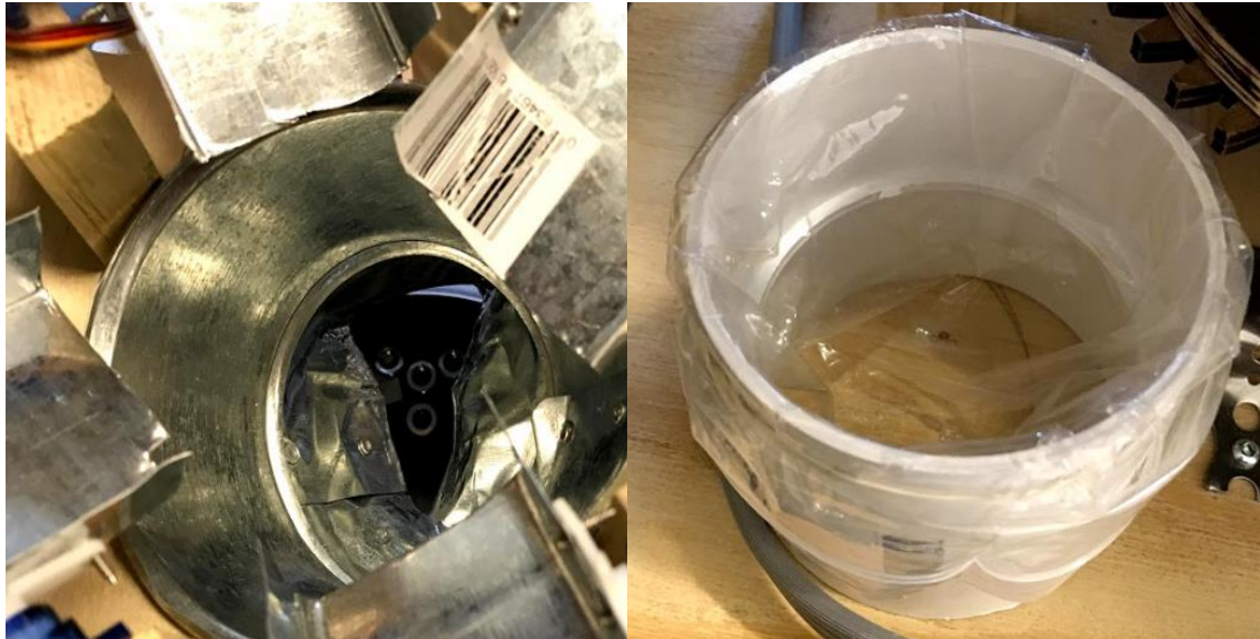
Figure 25 Funnel (directed to the opened fastener box) and Remaining Reservoir. Note that the open compartment is located directly below the exit of the funnel. Also note that there is a rubber band which tightens the plastic wrapper
