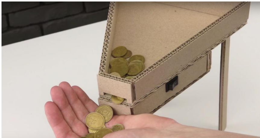
Figure 6 Vibratory Dispensing Machine [7]
